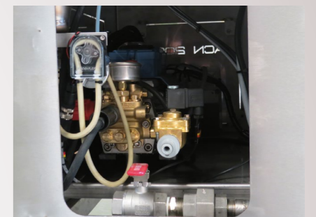
(1) Connection to the hydraulic network
